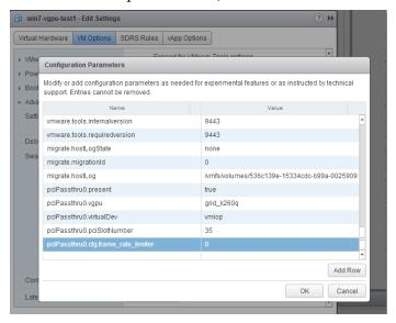
With this setting in place, the VM's vGPU will run without any frame rate limit. The FRL can be reverted back to its default setting by setting pciPassthru0.cfg.frame\_rate\_limiter to 1 or by removing the parameter from the advanced settings.
