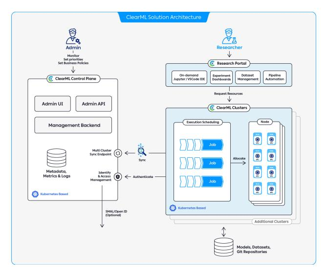
The ClearML installation consists of two components. The ClearML cluster (pictured above, right) and the ClearML Control Plane or Backend (left). Each of these components include options for how they can be deployed with the options being explained below.
